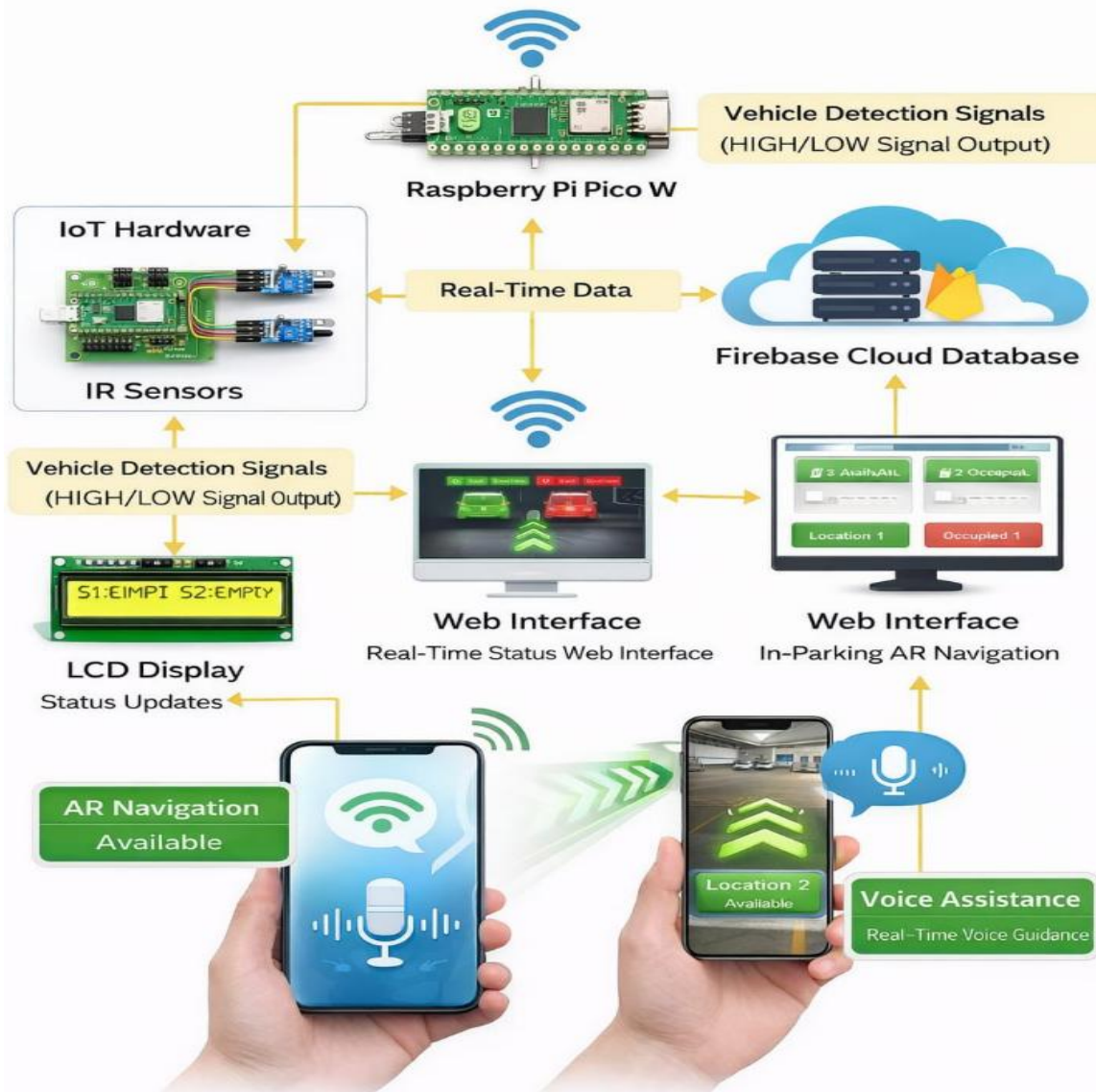
Figure 1: Architecture of the proposed IoT and AR-based smart parking system.
